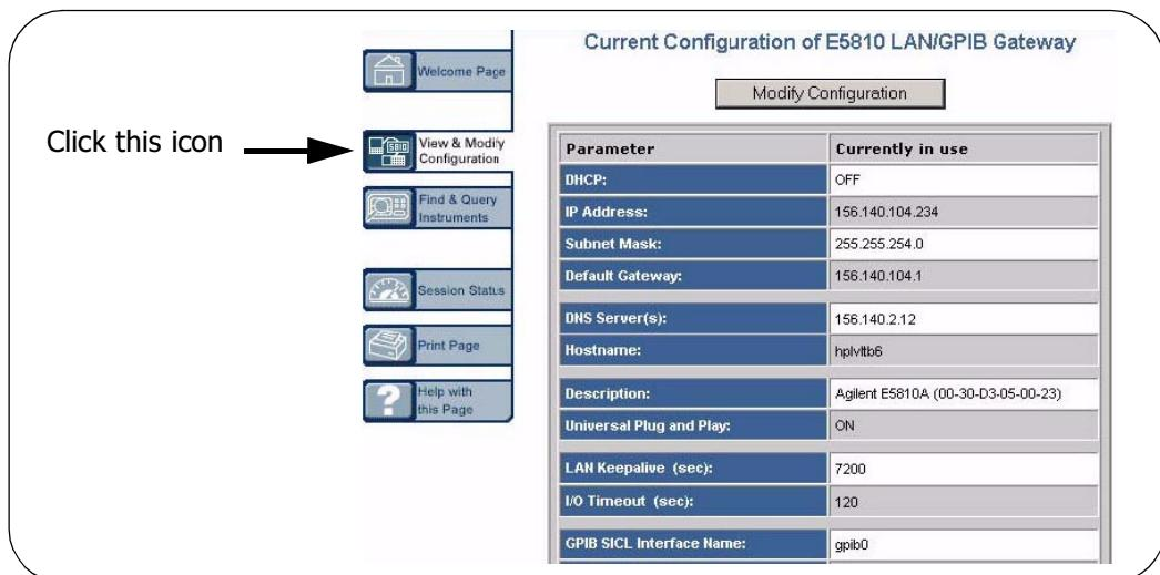
**3** **Display the Modify Configuration Page.** From the **Current Configuration of E5810 LAN/GPIB Gateway** page, click the **Modify Configuration** button to display the **Password** dialog box.
