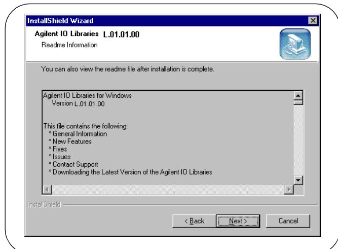
**8** Scroll through the **Readme Information** screen to display the latest Agilent IO Libraries information. When finished with the **Readme Information** screen, click **Next >** to display the **Select the Installation Option** screen. Click the **Full Installation** box and **Next >**.
