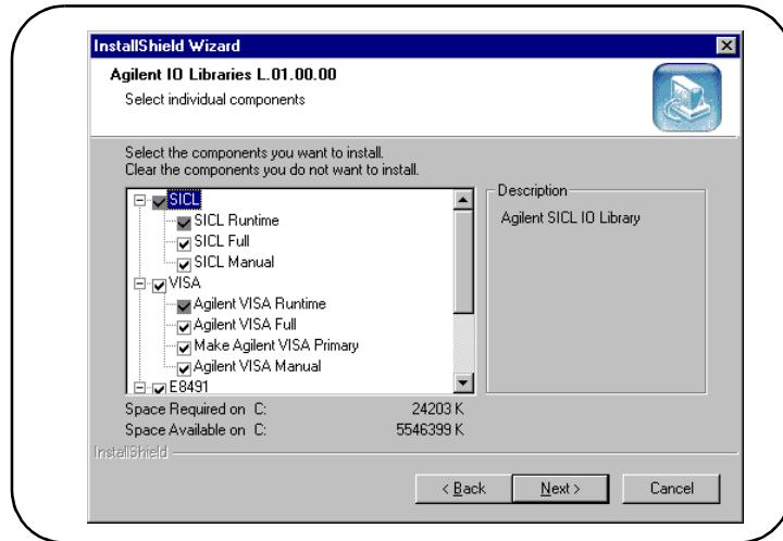
b Select the components you want to install and clear the components you do not want to install. Then, click **Next >** to display the **Current Settings** dialog box. This box shows the (default) paths in which VISA and SICL will be installed and the components that will be installed.
