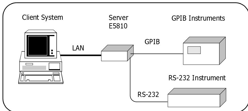
Thus, applications running on the computer system can transparently interface to GPIB and RS-232- based instruments over the LAN. Since several computer systems can access the E5810, groups of users can share access to the same GPIB and/or RS-232 instruments via the E5810. In addition, existing I/O applications that are supported with the E5810 and are designed for GPIB or RS-232 can use the E5810 without modification other than an address change.
