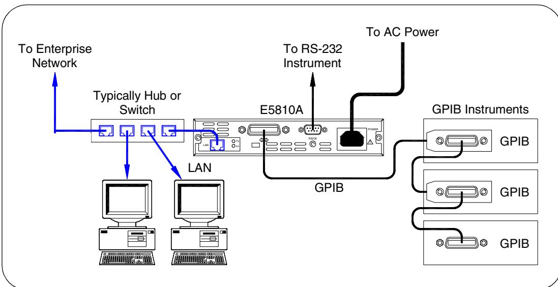
After connecting the E5810 to the Enterprise network, plug the E5810 AC power cord into an AC outlet and observe the power-on sequence. When the power-on sequence is complete, the assigned IP address of the E5810 is displayed on the second line of the front panel display. A typical display follows. See *Chapter 1 - E5810 Description* for power-on sequences.
