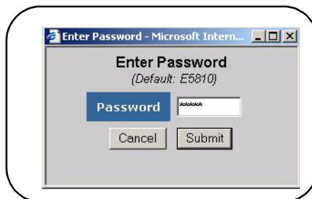
If the default password (E5810) is being used, the password is displayed as asterisks (\*\*\*\*). If not, type in the current password. Then, click the **Submit** button to display the **Configuring Your E5810 LAN/GPIB Gateway** page.
