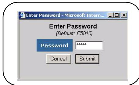
If the default password (E5810) is being used, the password is displayed as asterisks (\*\*\*\*\*). If not, type in the current password. Then, click the **Submit** button to display the **Configuring Your E5810 LAN/GPIB Gateway** page.
