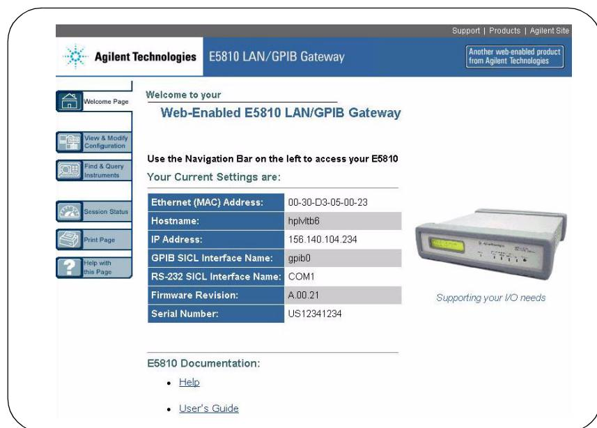
**2** **Display the Current Configuration Page.** from the **Welcome** page, click the **View & Modify Configuration** icon to display the **Current Configuration of E5810 LAN/GPIB Gateway** page
