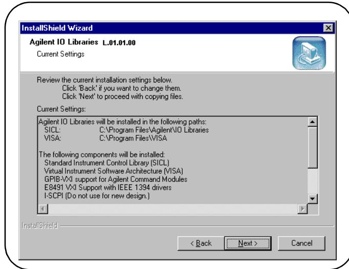
**10** Click **Next >** to accept the settings. Setup will then install the files and display the **Agilent IO Libraries have been successfully installed** screen. For E5810 installation, you can check the **Run IO Config** box if the E5810 has been installed and configured. (If desired, you can also check the **View Readme** box.)
